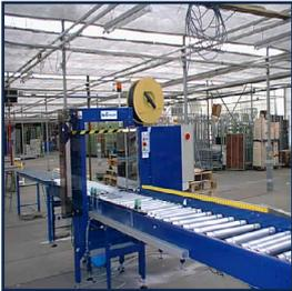
The CI 89 Y is a reliable automatic strapping machine, with a site seal. Because of the easy variety in strap tension (up to 800 N), the CI 89 Y is suitable for many different products. The automatic strapping machine CI 89 Y is available for many branches. This machine is perfectly suitable to build in automatic processing lines.
